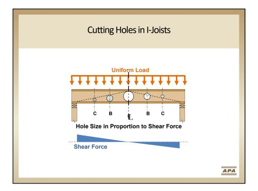
Near the bearing points, the shear forces are greatest. Generally holes in the web material can be larger the further they are from the I joists bearings.
